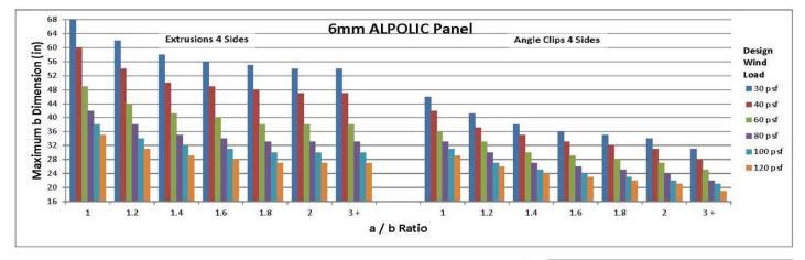
\* Controlled by maximum allowable bending stress (13,200psi) or maximum panel deflection (b/60) as applicable.
