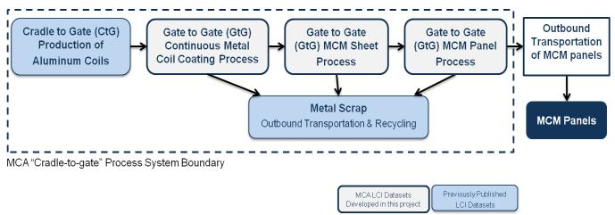
Figure 3: Cradle-to-Gate System Boundaries of MCM panels
