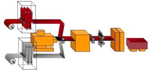
Figure 1: Schematic of MCM Laminating Process
